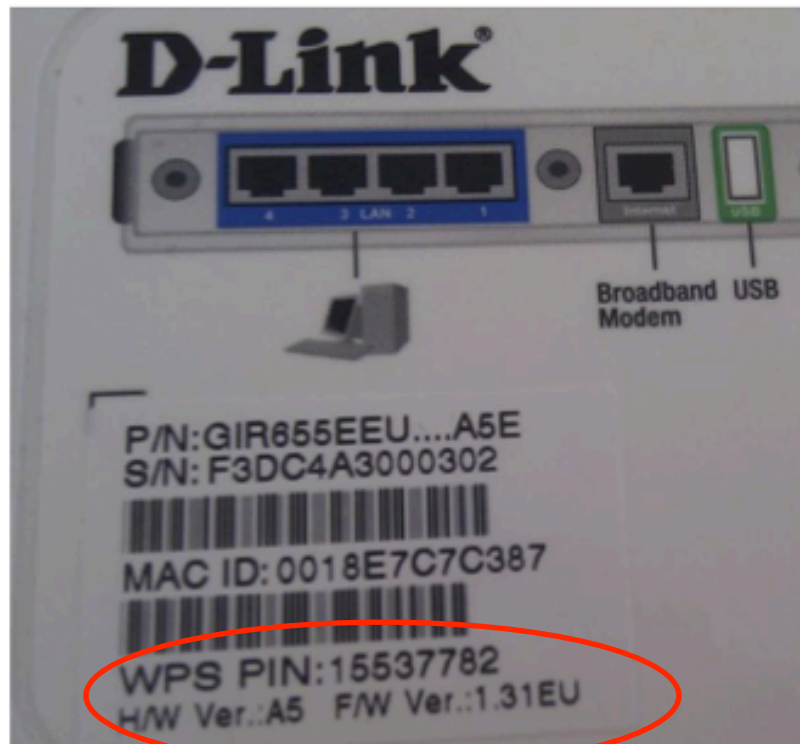
Figure 7: Label with WPS PIN on the back of a D-Link router
